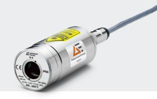
The Impac® IS 5 and IGA 5 are digital, compact, and fast infrared measuring instruments for non-contact temperature measurement on metals, ceramics, or graphite. For optimal match of the instrument to the application two optics with extremely small spot sizes are available.
