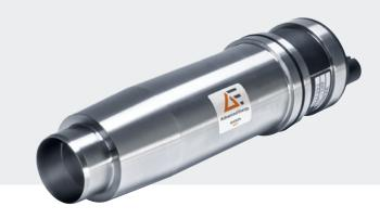
Completely self-contained, the Mikron® M67S infraducer can be used as true two-wire temperature transducer/transmitter which produces a standard 4 to 20 mA linear output. Powered by its current loop, each infraducer is completely compatible with any existing instrumentation for recording or process control.
