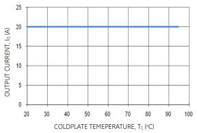
Figure 23. Derated Output Current versus Cold Wall Temperature with local ambient temperature around module at 85C;  $V_{\rm IN}$  =24V or 48V.
