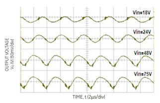
Figure 2. Typical output ripple and noise ( $I_0 = I_{0,max}$ ).
