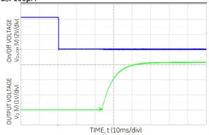
Figure 5. Typical Start-up Using Remote On/Off, negative logic version shown ( $V_{IN} = 24V$  or 48V,  $I_0 = I_{0,max}$ ).
