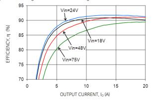
Figure 1. Converter Efficiency versus Output Current.
