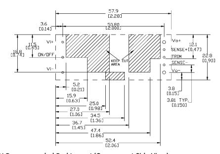
TH Recommended Pad Layout (Component Side View)
