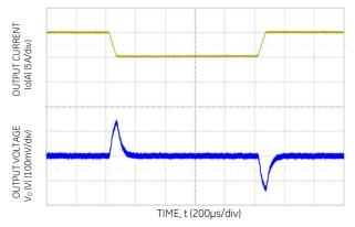
Figure 3. Transient Response to  $0.1A/\mu S$  Dynamic Load Change from 50% to 75% to 50% of full load, Vin=24V,  $C_0>100\mu F$ .
