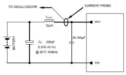
NOTE: Measure input reflected ripple current with a simulated source inductance (L<sub>TEST</sub>) of 12µH. Capacitor C<sub>S</sub> offsets possible battery impedance. Measure current as shown above
