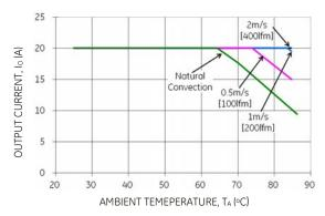
Figure 21. Output Current Derating for the Module with-18 Heatplate; Airflow in the Transverse Direction from Vout(-) to Vout(+);V<sub>IN</sub> =24V.
