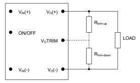
Figure 12. Circuit Configuration to Trim Output Voltage.
