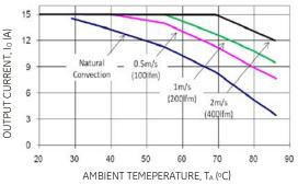
Figure 16. Output Current Derating for the Open Frame Module (including the –D option); Airflow in the Transverse Direction from  $V_{out}$ (-) to  $V_{out}$ (+);  $V_{IN}$  =48V,  $V_0$ =5.0V.
