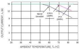
Figure 21. Output Current Derating for the Module with -18 Heatplate; Airflow in the Transverse Direction from  $V_{out}(-)$  to  $V_{out}(+)$ ; $V_{IN} = 24V$ ,  $V_{O} = 5.0V$ .
