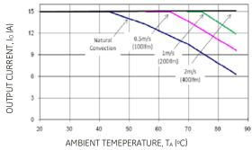
Figure 20. Output Current Derating for the Module with Heatplate; Airflow in the Transverse Direction from  $V_{out}(-)$  to  $V_{out}(+)$ ; $V_{IN} = 24V$ ,  $V_0 = 5.0V$ .
