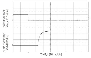
Figure 5. Typical Start-up Using Remote On/Off, negative logic version shown ( $V_{IN} = 48V$ ,  $I_0 = I_{0,max}$ ).
