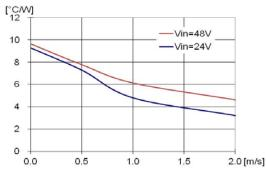
Figure 15. Thermal Resistance for the Open Frame Module; Airflow in the Transverse Direction from V<sub>out</sub>(-) to V<sub>out</sub>(+); V<sub>IN</sub> =24V or 48V, V<sub>0</sub>=5.0V.
