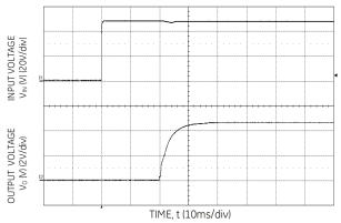
Figure 6. Typical Start-up Using Input Voltage (VIN = 48V, Io = lo,max).
