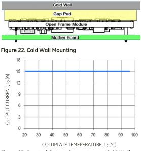
Figure 23. Derated Output Current versus Cold Wall Temperature with local ambient temperature around module at 85C;  $V_{IN}$  =24V or 48V.
