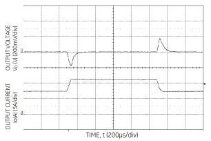
Figure 3. Transient Response to 0.1A/µS Dynamic Load Change from 50% to 75% to 50% of full load, Vin=24V, Co>100µF.
