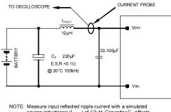
source inductance (L<sub>TEST</sub>) of 12µH. Capacitor C<sub>s</sub> offsets possible battery impedance. Measure current as shown above.
