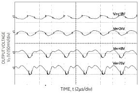
Figure 2. Typical output ripple and noise  $(I_0 = I_{0,max})$ .
