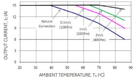
Figure 19. Output Current Derating for the Open Frame Module; Airflow in the Transverse Direction from  $V_{out}$ (-) to  $V_{out}$ (+);  $V_{IN} = 24V$ ,  $V_0 = 5.0V$ .
