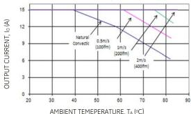
Figure 18. Output Current Derating for the Module with -18H Heatplate; Airflow in the Transverse Direction from  $V_{out}(-)$  to  $V_{out}(+)$ ; $V_{IN} = 48V$ ,  $V_0 = 5.0V$
