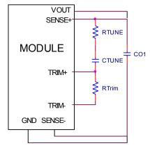
Figure. 28. Circuit diagram showing connection of  $R_{\text{TUNE}}$  and  $C_{\text{TUNE}}$  to tune the control loop of the module.
