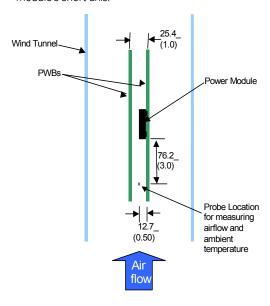
Figure 29. Thermal Test Setup.
