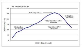
**NOTE:** Soldering outside of the recommended profile requires testing to verify results and performance.
