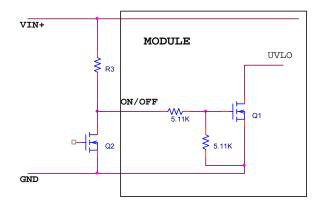
Figure 24. Circuit configuration for using negative On/Off logic.
