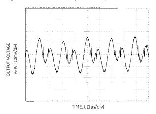
Figure 9. Typical output ripple and noise ( $V_{IN}=12V_{t}$ ,  $I_{o}=I_{o,max}$ ).
