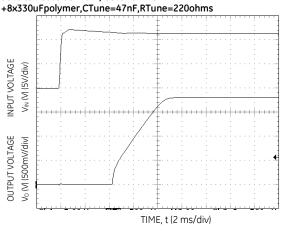
Figure 18. Typical Start-up Using Input Voltage ( $V_{IN} = 12V$ ,  $I_0 = I_{0,max}$ ).
