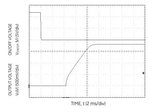
Figure 17. Typical Start-up Using On/Off Voltage ( $I_0 = I_{O,max}$ ).
