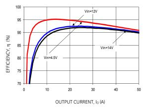
Figure 13. Converter Efficiency versus Output Current.
