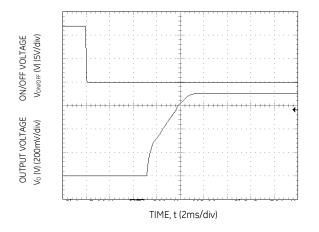
Figure 5. Typical Start-up Using On/Off Voltage ( $I_0 = I_{0,max}$ ).
