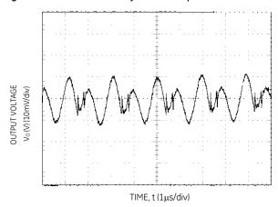
Figure 3. Typical output ripple and noise ( $V_{IN} = 12V$ ,  $I_0 = I_{O,max}$ ).
