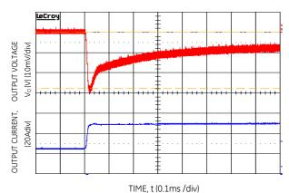
Figure 10. Transient Response to Dynamic Load Change from 50% to 100% at 12Vin, Cext =5x47uF+
