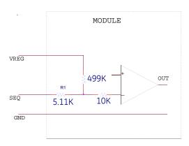
Figure 27. Circuit showing connection of the sequencing signal to the SEQ pin.
