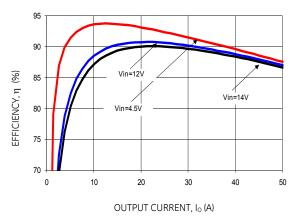
Figure 7. Converter Efficiency versus Output Current.
