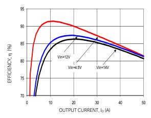
Figure 1. Converter Efficiency versus Output Current.
